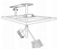
Figure 2 Three-dimensional model of the brushing unit
